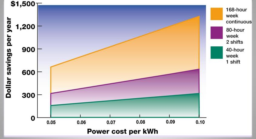
40 HP Super-E with 94.5% efficiency compared to standard motor with 90% eff.Operating 50 weeks/year
